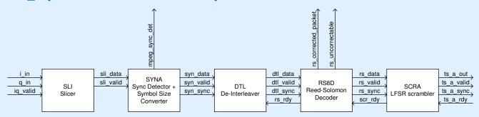
The DEC\_A sub-block supports the full set of DVBC constellations, of which J.83 Annex A and C are subsets. This includes 16-, 32-, 64-, 128- and 256-QAM.
